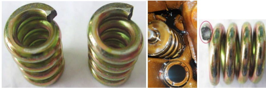
Fig. 2. Broken exhaust valve spring
