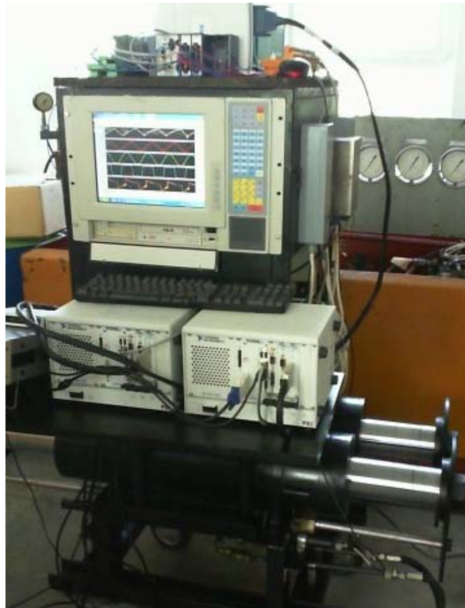
Fig. 12. Functional speed governor model using NI cRIO technology
