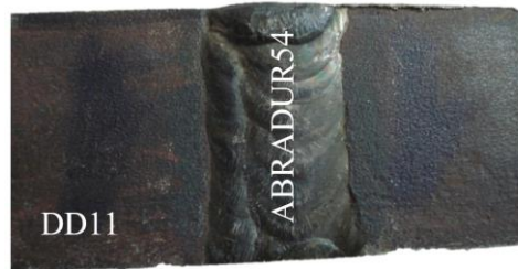
Fig. 1. DD11 steel hardfacing welded with ABRADUR54 electrode
