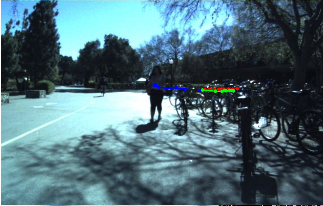
Fig. 3. Result example of the of People Trajectory Prediction module. The blue line represents the previous observed trajectory, the red line represents the estimated future trajectory predicted by the module based on the observations and the green line represents the real trajectory followed by the person.
