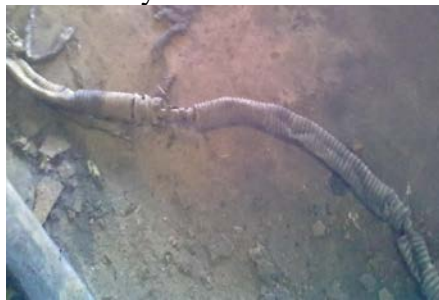
Fig. 12 Damaged cable of ejector motor
