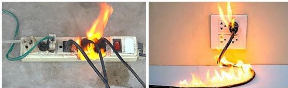
Fig. 6 Fire caused by imperfect contacts and overload.
