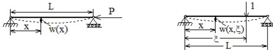
Fig. 2. Buckling of a pin-ended straight beam and the corresponding Green function
