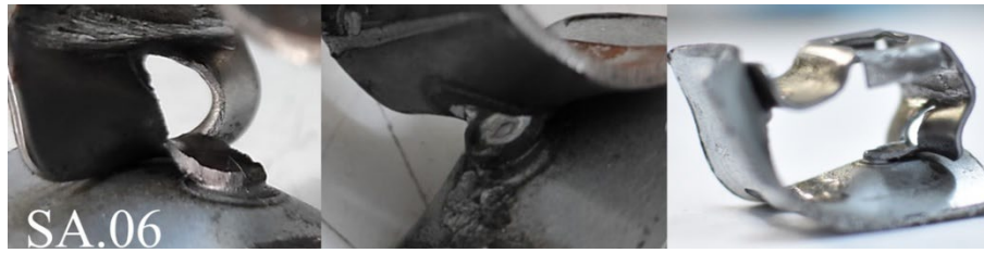
Fig. 14. Failure of samples observed in chisel-test (manual destruction test)
