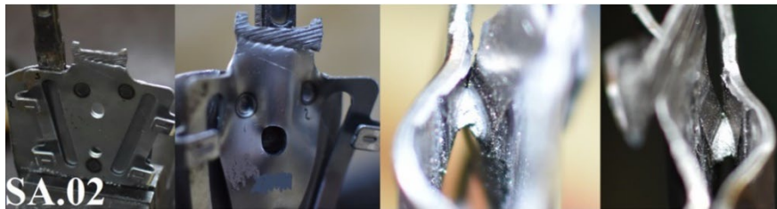
Fig. 12. Failure of samples observed in chisel-test (manual destruction test)
