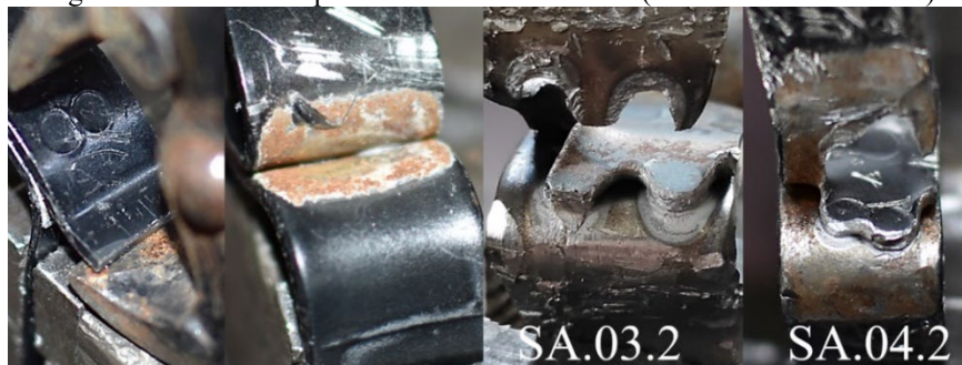
Fig. 13. Failure of samples observed in peel-test (manual destruction test)
