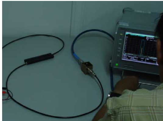
Fig. 10. The test assembly used for the \Pi matching circuit's adjustment.
