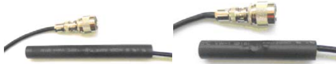
Fig. 8b. Antennas for 450 MHz and for 750 MHz with thermo-contraction protection tube.
