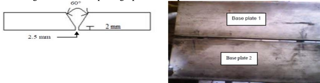
Fig. 1. Block diagram of joint design and Base metal Positioning
