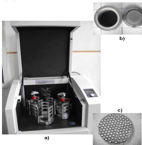
Fig. 1. a) High energy planetary mill RETSCH PM400; b) Milling vial; c) Milling balls
