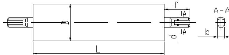
Fig. 7 Design parameter diagram of central roller shaft
