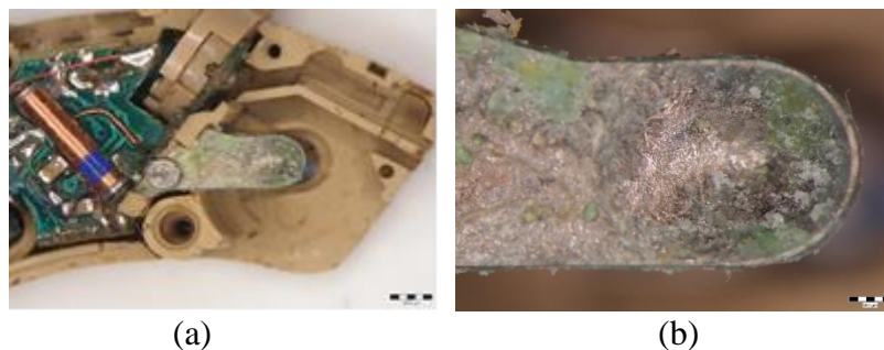
Fig. 1- Stereomicroscopic images of the hearing aids: a-position of the lamella in the hearing aid; b- macroscopical aspect of hearing aid contact lamella
