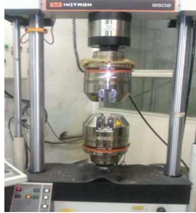
Fig.3. INSTRON 8502 servo hydraulic machine.
