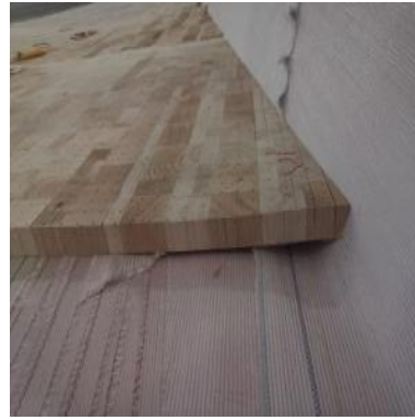
Fig. 9 Layering with gaps
