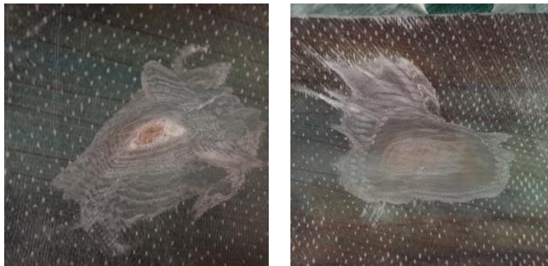
Fig. 11 Schematic diagram of defect grinding
