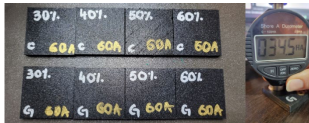
Fig. 9. Filaflex 60A – samples and measurement with Shore A durometer
