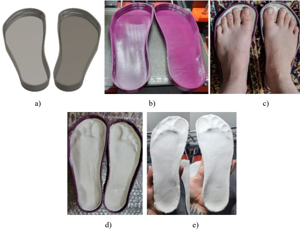
Fig 8. Peak plantar pressure evaluation process: a) 3D modeling the molds; b) 3D-printed molds; c) Clay forming; d) Baking ready molds; e) Fully hardened clay.
