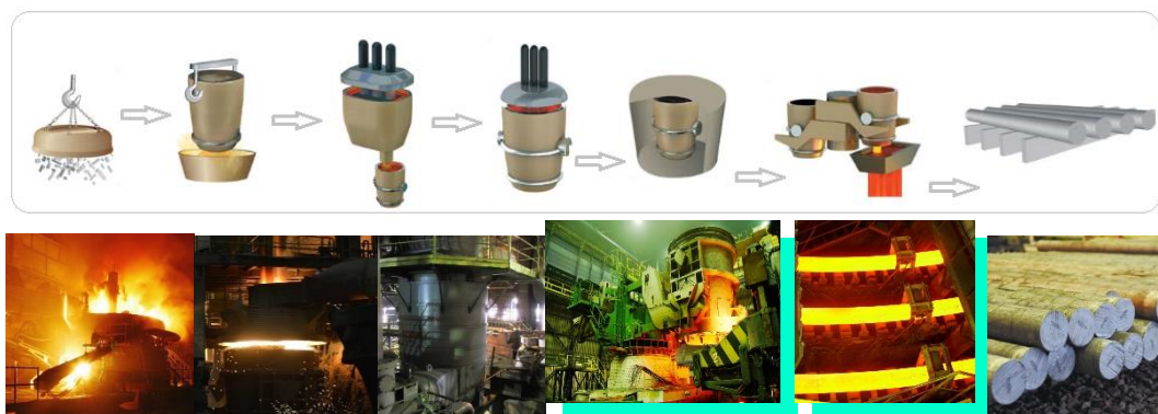
Fig. 2. The technological flow of steel production
