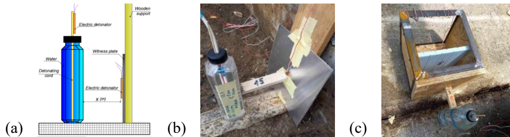
Fig. 5. (a, b) Configuration used for determining the minimum distance for positioning the neutralization charge relative to the (IED); (c) Testing configurations for assessing the material behavior
