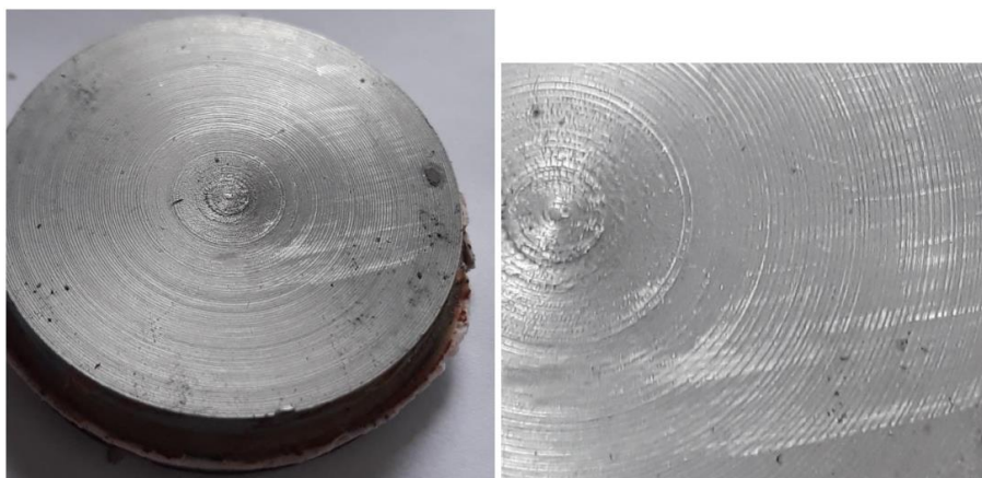
Fig. 7. a) Wear appearance on the control sample surface M.1; b) detail of the trace produced by the surface abrasion erosion test M.1.
