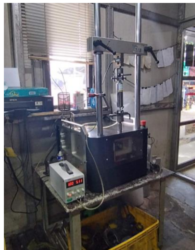
Fig. 9. Experimental setup using damper dynamometer
