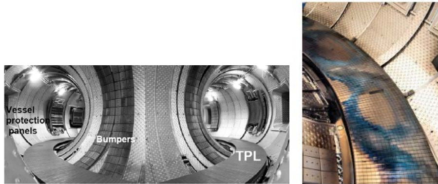
Fig 1: Panoramic view of Tore Supra CIEL configuration (left). TPL image showing erosion and co-deposits areas (right) [6]
