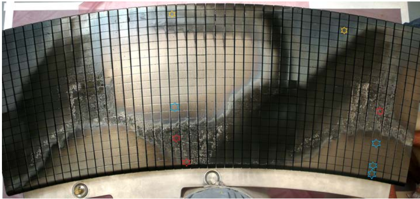
Fig. 2: The LPT of Tore Supra after plasma discharges. Stars are indicating the location from where the sampling was done. Blue, red and yellow stars marked the erosion area, thick deposition and respective, thin deposition.
