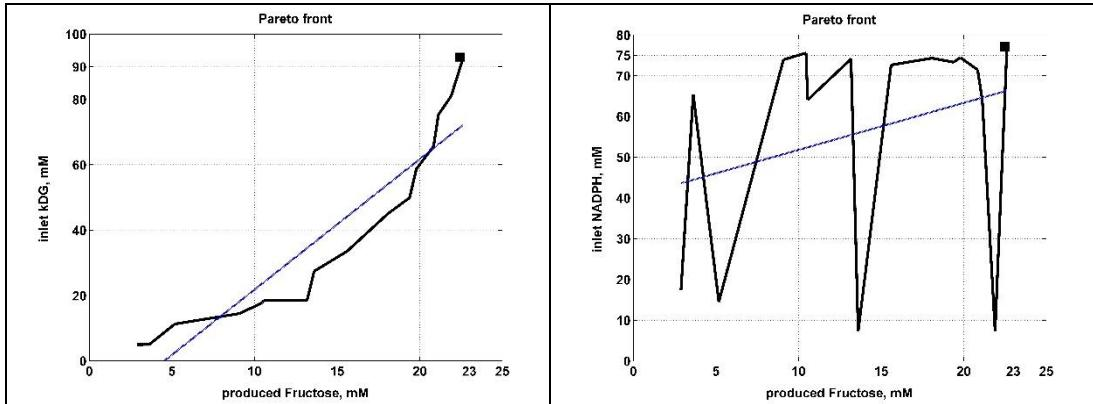
**Fig. 4.** The Pareto-optimal front in terms of Min. substrate (kDG) consumption (initially added)-vs.- Max. P(D-fructose) production, for **OWL** limits (**Table 1**) of control variables. The marked SP was chosen according to [63-67]. The blue line is the smoothed Pareto-optimal front.
