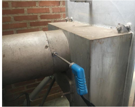
Fig. 3.2. Positioning of the flue gas analyzer probe in the flue gas channel connecting the boiler to the chimney
