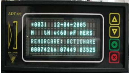
c. Intelligent display information main menu with action to take, line 3 “TRACKING “ of the vehicle to depot
