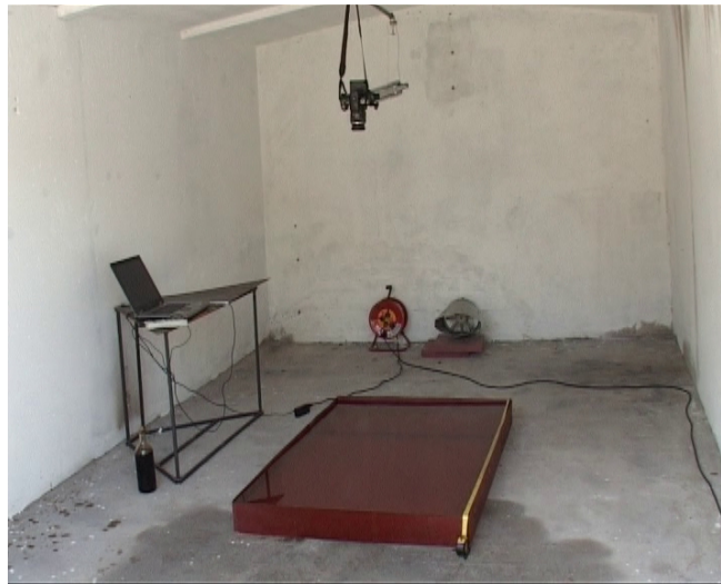
Fig. 1. Experimental laboratory stand used to visualize an oil spill on the water surface
