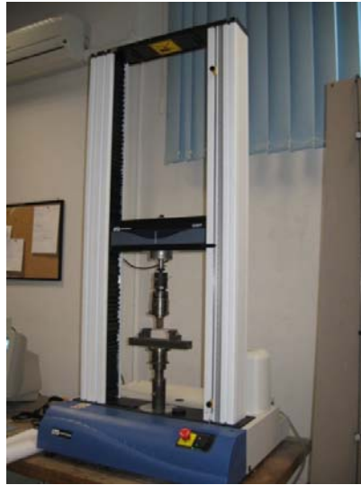
Fig.2. Test bench used in the three-point bending tests.
