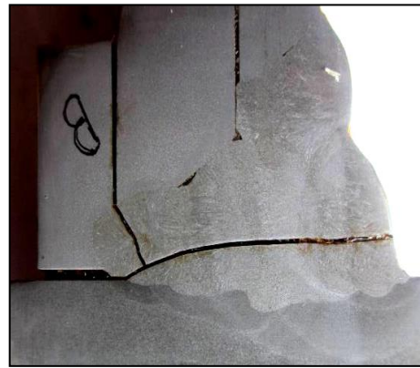
Fig. 3. Fatigue Failure of Doubler Plate
