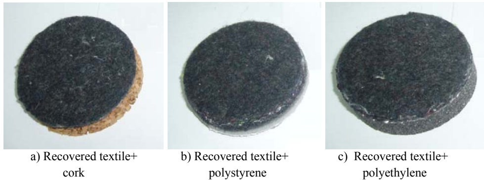
Fig. 1. Variants of multi-layered composite materials undergoing tests
