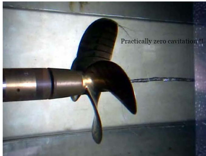
Fig. 8. Simulated nominal wake testing, in 850x850 mm section of the cavitation tunnel at 25 rps rotative speed (it can be remarked lack of cavitation).
