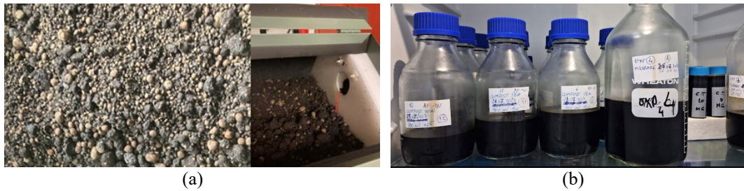
Fig. 1. Compost obtained in the compost tumbler by composting rockweed ( A. nodosum ) residues with LECA (lightweight expanded clay aggregate) and granulated sugar (a) and related non-aerated compost tea (CT) (b).
