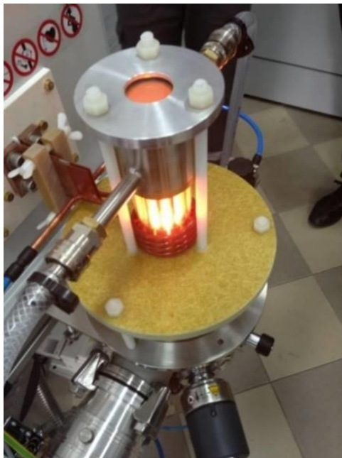
Fig.1. Induction furnace with cold crucible, vacuum and argon atmosphere
