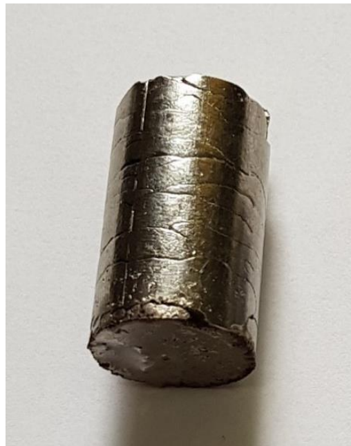
Fig.2. Shape of the stainless steel ingot produced in the induction furnace with cold crucible
