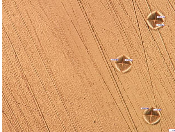
Fig. 9 Vickers micro-hardness imprints on the Ag coating
