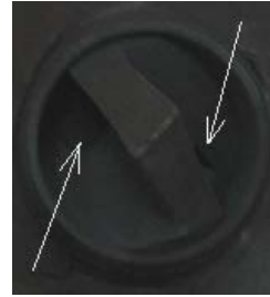
Fig.3. Detail (inlet of the cooling primary agent in the nozzle)
