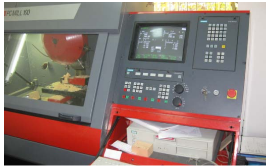
Fig. 8. Machining the vertebra on EMCO PC MILL 100
