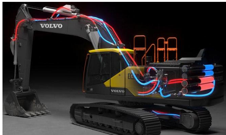
Fig. 33. The world's first all-electric excavator with energy recovery system by electrohydraulic servomotors based on DANFOSS digital pumps (VOLVO)
