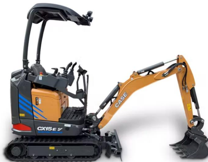
Fig. 6. Electrohydraulic CASE CX15 EV mini excavator powered by a 16 kW electric motor and 21.5 kWh lithium-ion battery [3]
