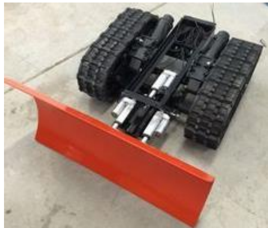
Fig. 31. Snow plough with electric propulsion and hybrid actuators for the front blade
