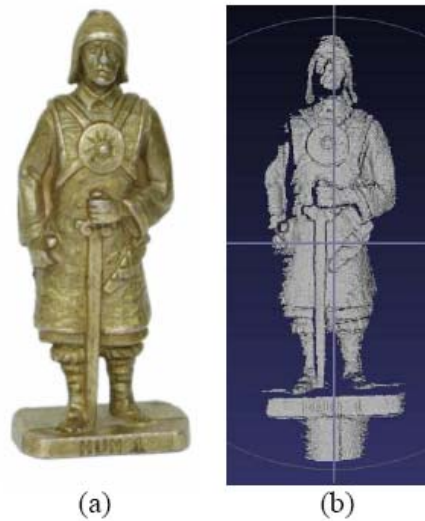
Fig. 9 Laser scanner resulted 3D data. Original part (9a) and resulted point cloud (9b)
