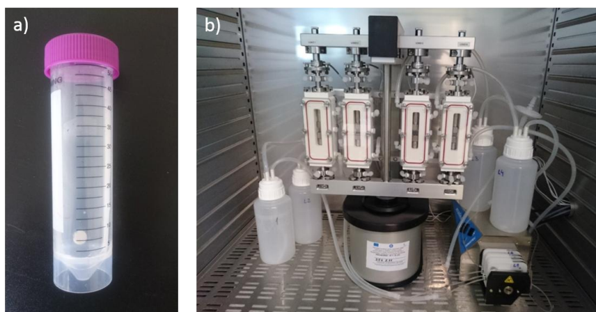
Fig.1. Representative experimental set-up:a) Conventional vial with SBF-incubated sample, b) ElectroForce 5210 biodynamic test instrument
