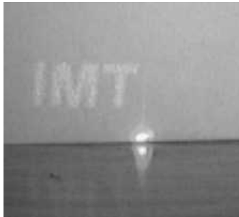
Fig. 7. The far-field image obtained with the fabricated DOE
