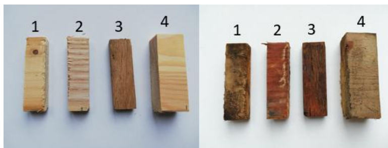
Fig. 1 Wood before (left) and after aging (right): 1 - fir, 2 - ash, 3 - oak, 4 - pine
