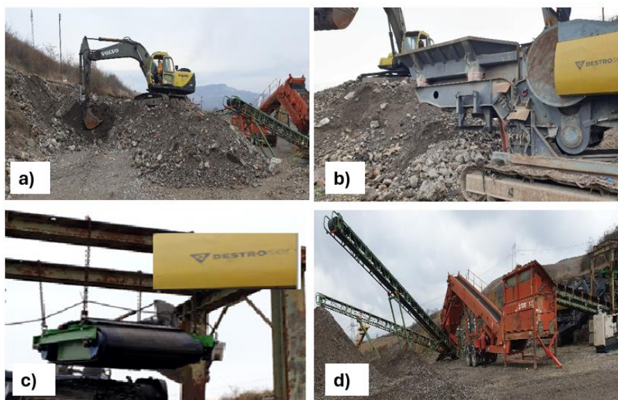
Fig. 6. The main steps of the DESTRO comminution technology applied at Călan landfill: a) wastes gathering; b) crushing step; c) magnetic deferrization; d) sieving and sorting stage.
