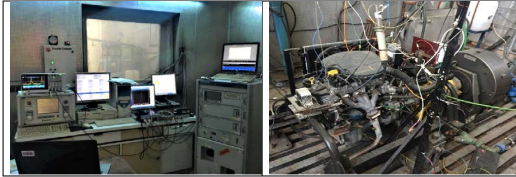
Fig. 1. The engine test cell with the control room and the test bench
