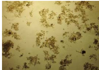
Fig. 6a – Microscopic image of the activated sludge – general image (40x)
