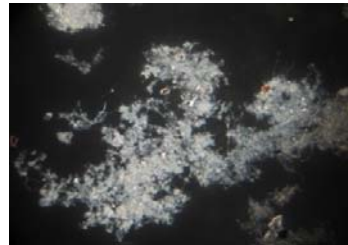
Fig. 6b - Microscopic image of the activated sludge – detailed flocs (100x)
