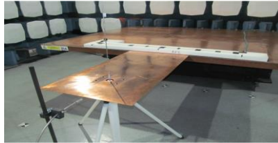
Fig. 1. Radiated emissions. Experimental test setup and Feko simulation model geometry
