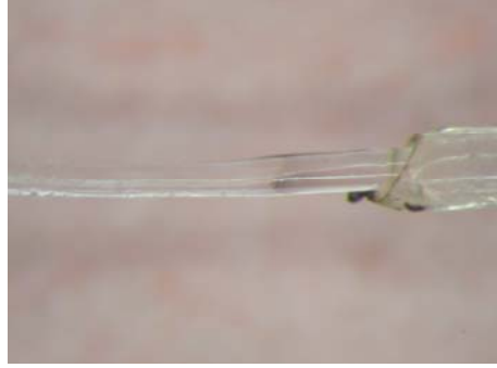
Fig. 5. The image of the damaged optical fiber at a scanning speed of the laser less than v = 0.6 \text{ m/min} .
