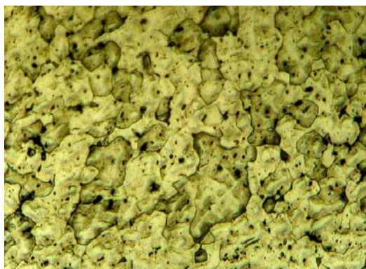
Fig. 2 As-cast alloy structure; Transversal section; Original magnification: x250
