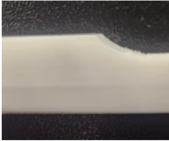
Fig.5. Fourth PLA object with defects on the surface
