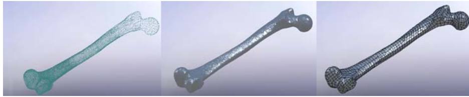
Fig. 5. 3D reconstruction of femur using ScanTo3D software module from SolidWorks
