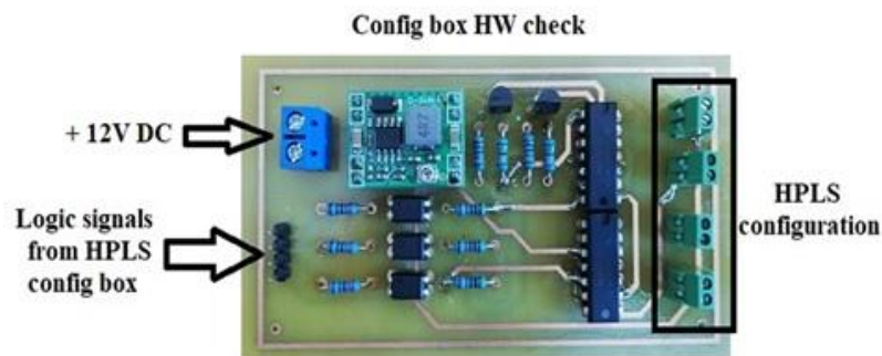
Fig. 5. PCB for configurator box hardware check electronic module
