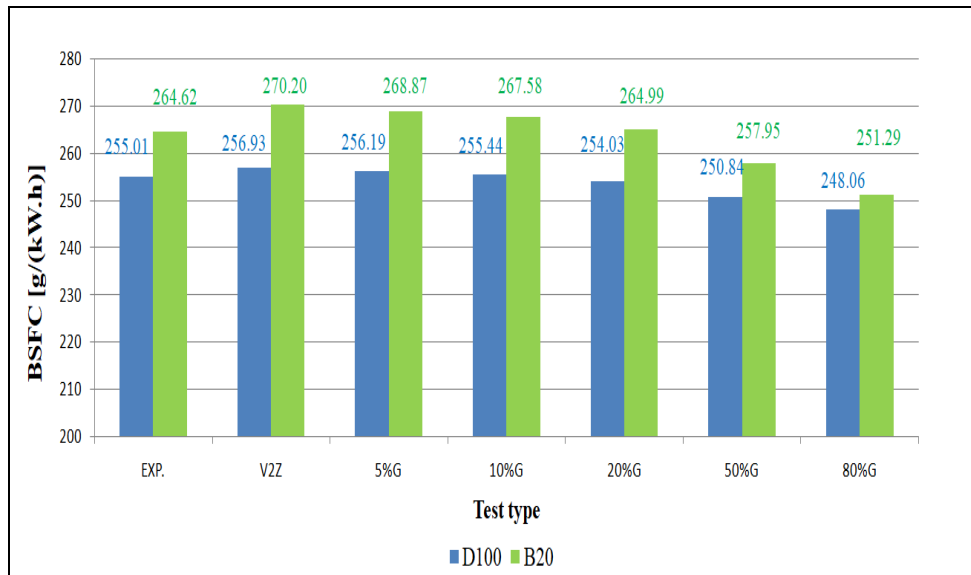
Fig. 9-BSFC results from experiment and simulation for different tested fuels
