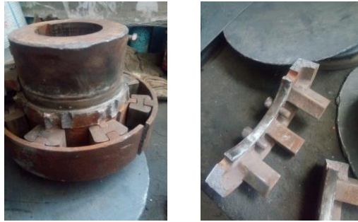
Fig. 2 The damaged mechanical coupling of a 6 kV, 200 kW induction motor driving an exhauster due to unsuccessful DLT.
